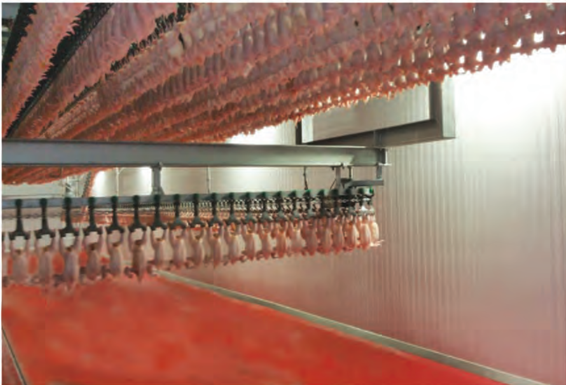
Fully hygienic carcass chilling to 1,5°C
