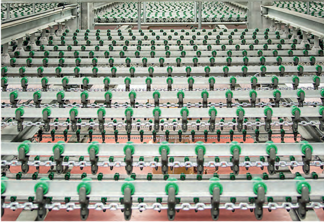
Chilling line chain ca. 6,2 km long
